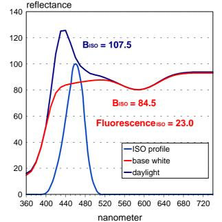
Figure 5. Separation of base white from total reflectance spectrum showing individual brightness contributions.
