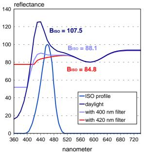
Figure 4. Reflectance values under different UV filters
